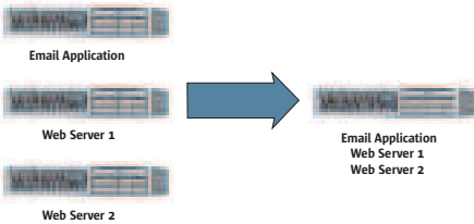
Figure 1—With server virtualization, applications can be safely consolidated onto a fewer number of servers.
